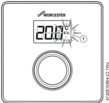
Fig. 22 Low battery indication
